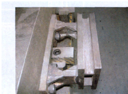
图 11 焊接形式的侧模瓣侧拉块 Fig.11 Welded die flap and pulling chip on the side of the mold
